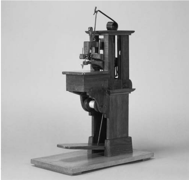
Barthélemy Thimonnier sewing machine (Sewing Machine - Barthélemy Thimonnier - Google Arts & Culture, n.d.).
