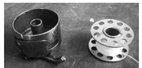
Bobbin and bobbin case for a shuttle hook sewing machine, introduced by Singer for the "Improved Family" model in 1895 (Wikipedia, 2023).
