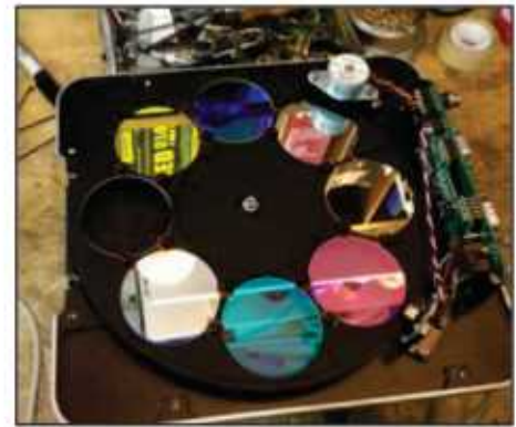
Filter Wheel for Yerkes 41-inch Telescope
