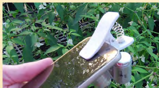
Figure 12. Using a smartphone with a clip-on lens to take photos of insects (Photo credit: B. Liedl).
