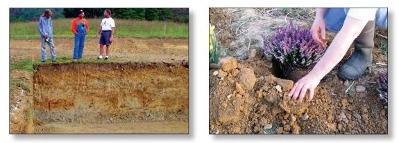
Exposing the soil profile and evaluating the soil before building will provide property owners and builders with an understanding of whether the soil is suitable for lawns and gardens, foundations, and on-site wastewater treatment systems.
