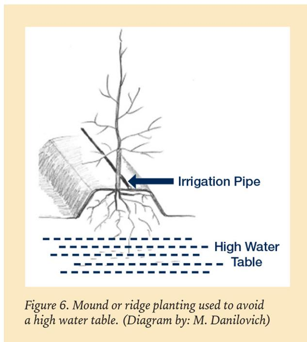
Figure 6. Mound or ridge planting used to avoid a high water table. (Diagram by: M. Danilovich)
