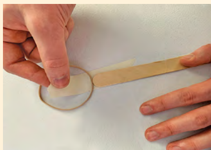
Figure 5. Fold double layer of tape over rubber band and onto craft stick to make launcher.
