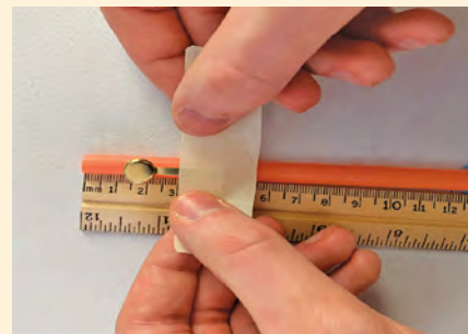
Figure 3. Metal fastener should be approximately 1 cm from top edge of straw.
