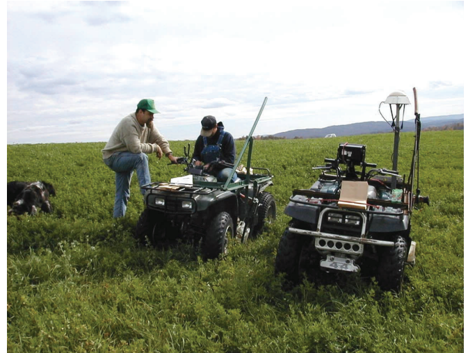
Figure 1 - Soil Sampling with GPS Referencing This geo-referenced soil fertility information is then used to apply variable rates of nutrients or lime to a field.
