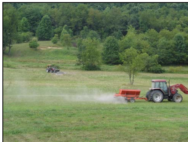
Figure 4. Lime can be spread at any time during the year, but late summer and fall are often good times to apply lime. Lime spreaders apply lime evenly over the soil. Some spreaders are pulled by a tractor, while other spreaders may be mounted directly on trucks.
